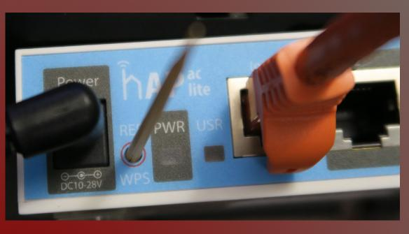
Press and hold the reset button on the node while powering on the PoE unit or the device.
