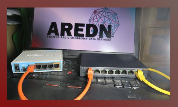
With the PoE unit powered off, connect the Mikrotik node to the POE port.
