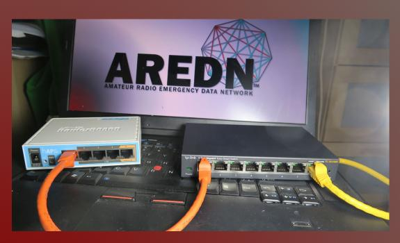
Do "ping" on 192.168.88.1 w/this cable from setup to verify HAP is on 88.1 and Mikrotik to not 1.1 do not proceed until you have a good ping.
